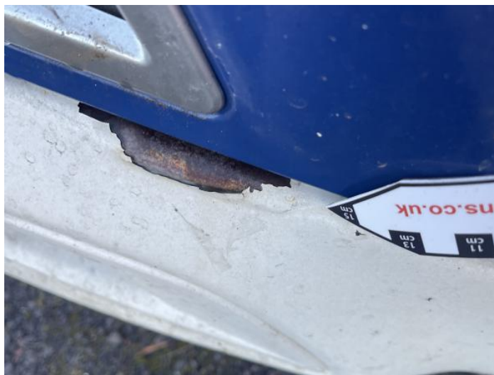
2: Bumper Front Rusted Over 5mm
